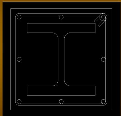
Shape Min. dim. no steel 39x39 W12x17036x36 W12x210 35x35 W12x230 35x35 W14x257 33x33 W14x311 31x31 W14x500 23x23
